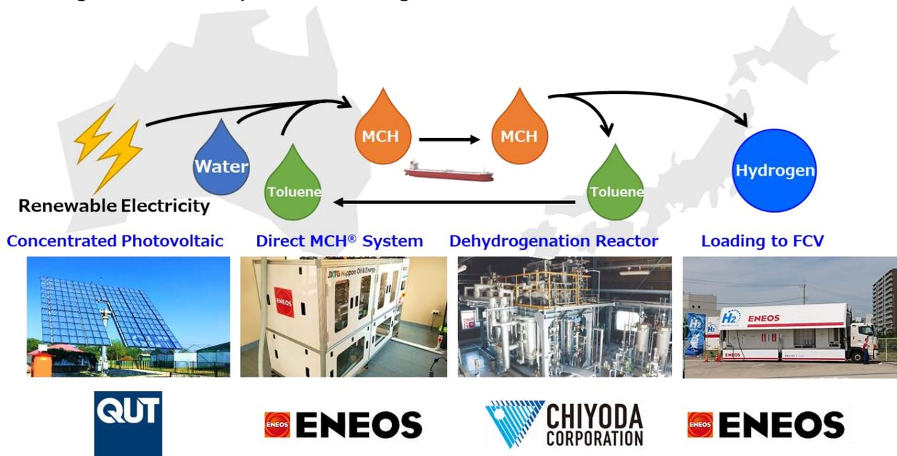
1. QUT generates power using its Concentrated Photovoltaic Power Generation System
